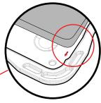
B If latch does not operate smoothly or securely, repeat step #3 to ensure fitment.
