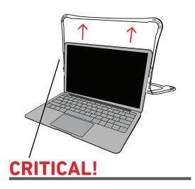
The monitor must be SLID out of the case. Failure to do so through forecefully popping/pressing the monitor out may cause damage to the device.
