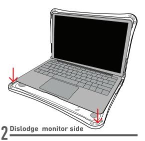
Use your fingers behind the hinge of the device/case to slide the case up a few inches to dislodge it.
