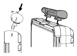
To remove the stylus holder, tilt the front and pull up and away.
