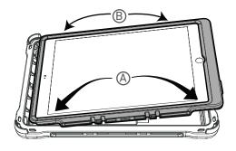
BInsert the remaining top 2 edges (the LATCH side) into the outer case.
