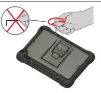
5 Use included hex tool to tighten 4 screws by rotating clockwise until snug. DO NOT over tighten.
